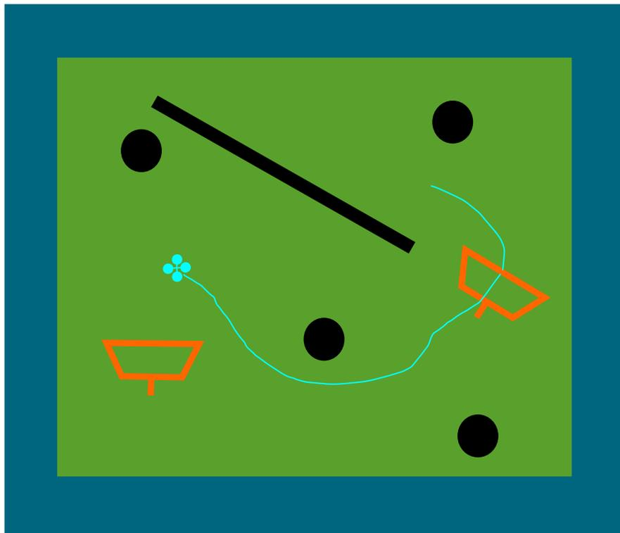
**Illustration of the competition.** The tiny blue drone needs to avoid obstacles and fly as fast as possible to cover as much distance as possible within the arena (green area). It can gain extra points by passing through orange gates. We are currently planning to fly in a 10 x 10 m arena, where the drone should stay in an inner 8 x 8 m area. The video shows the arena, the “Cyberzoo”.
